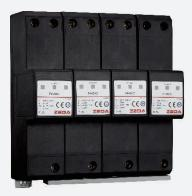
DIN rail, combined Type 1&2 / Class I&II with MOV and CDGG technology for use in TN-C system at boundaries from LPZ 0a-2
