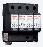
DIN rail, Type 2 / Class II multi-purpose SPD with anti-vibration pluggable module for use in TN-S or TT system at boundaries from LPZ 0<sub>8</sub>-1 and higher.
