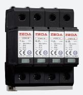
DIN rail, Type 2 / Class II multi-purpose SPD with anti-vibration pluggable module for use in TN-S or TT system at boundaries from LPZ 0<sub>8</sub>-1 and higher.
